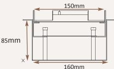
Frame size 150x150mm Base box size 160x160mm
