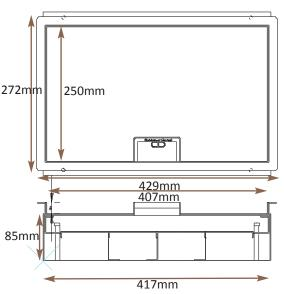
Frame size 407x250mm (plus visible trim flange 12.5mm) Base box size 417x260mm
