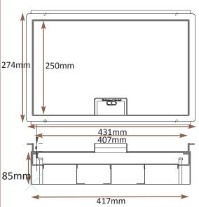
Frame size 407x250mm (plus visible trim flange 12mm) Base box size 417x260mm Lid recess - advise on order to suit floor covering Base with 20 & 25mm conduit knockouts in base and sides
