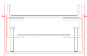
Standard floor box with fixing flange (base box installed BEFORE final floor is fitted)
