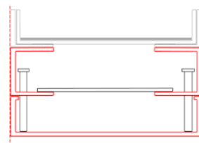
Retrofit floor box without fixing flange (floor box installed AFTER final floor is fitted or with a poured finish, i.e. terrazzo/polished screed)
